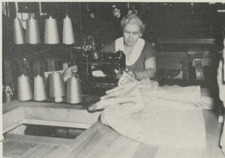
SADIE SHELTON of the Binding department, a veteran of 24 years, is shown as she quickly and expertly stitches a satin ribbon on the wooly blankets. (Staff Photo)
