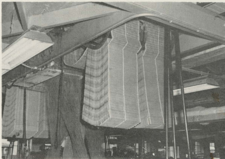
THE CARDS AND CORDS shown above compose the Jacquard head that controls the patterns to be woven. Practically any design can be made with this complicated mechanism. (Staff Photo)
