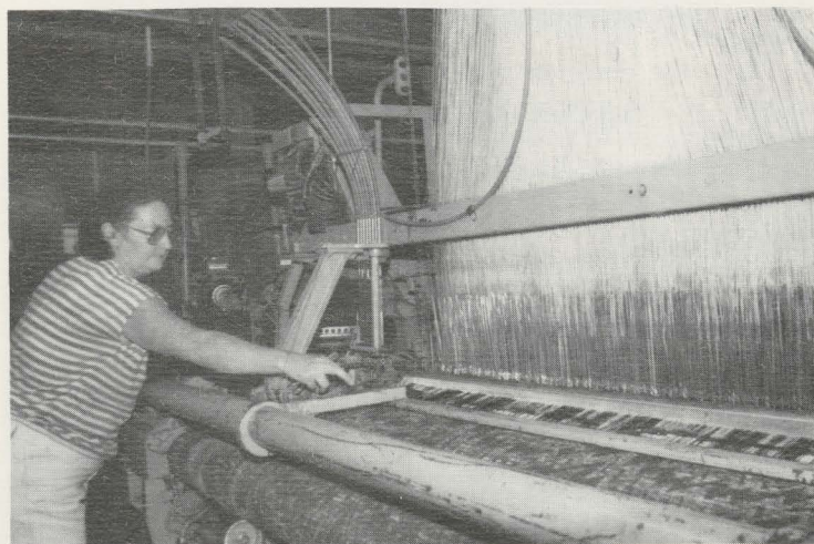
Linda Thomas, Weave Department employee, checks on the Jacquard loom as the material is woven. Jacquard ties flow down to the weave machine from the Jacquard head: This particular pattern has 4,536 cords coming down and the pattern controls the movement of each cord.
