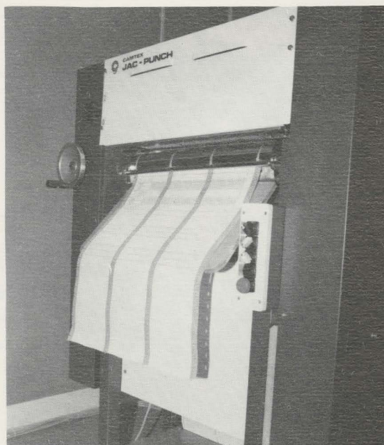
A Jacquard pattern emerges from the Jac-Punch machine.
