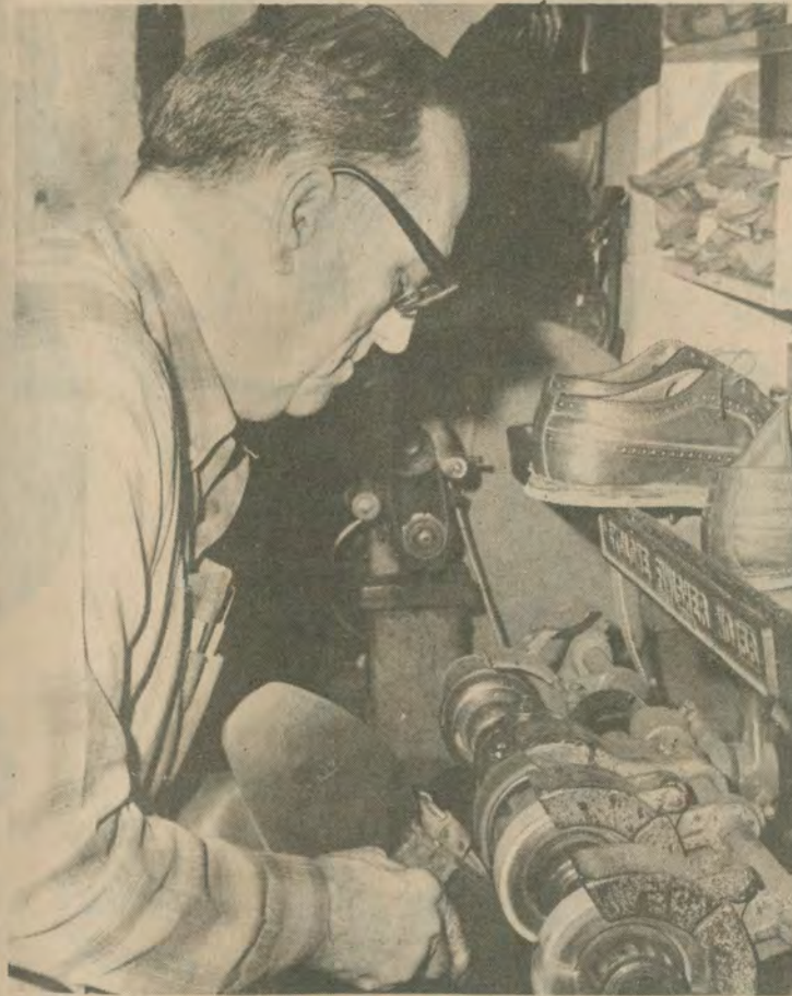
SANDING the edge of a new heel, Davis uses equipment that may be older than he is. He says he really doesn't know how old the machines are—at least 50 years—but they do the job.
