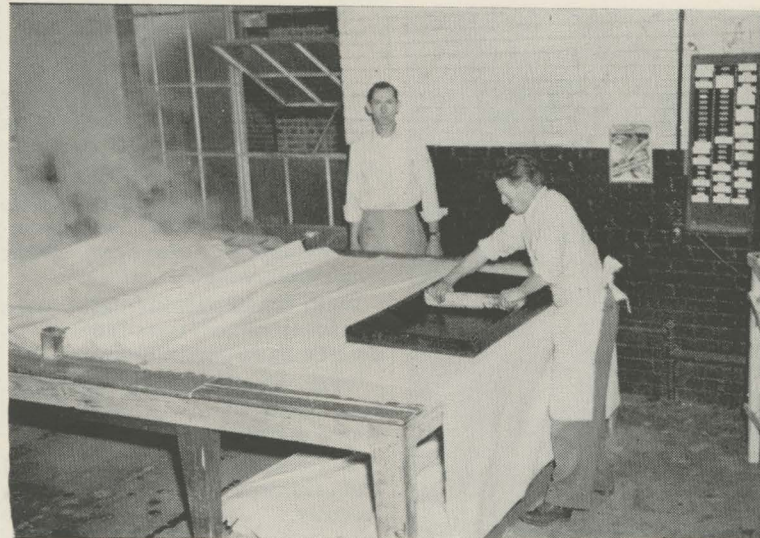
THE SCREEN PRINTING CREW — Jodie Mathis, right and Ernest Edwards, are seen engaged in printing a name or monogram on hundreds of woolen blankets for some hotel, hospital, steamship company, etc. The cloud of steam in the background comes from the steaming operation that "sets" or fastens the color of the printed name more or less permanently into the fabric. (Staff Photo)
