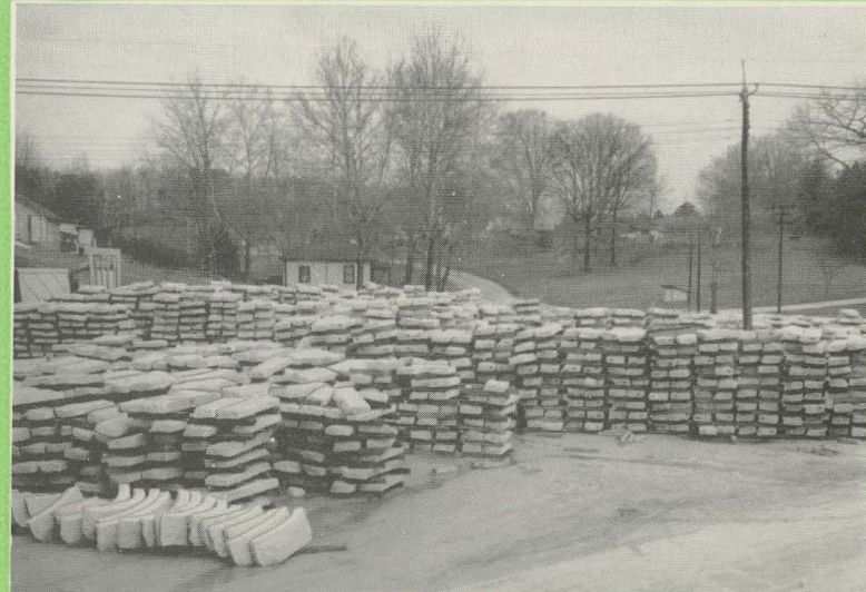
Stock Pile of Vertical Curbing with Sloped Face
