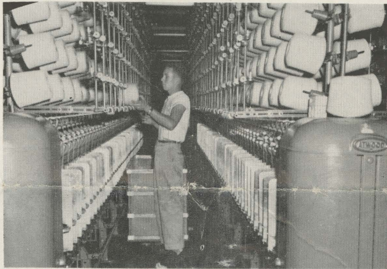
WARNER HOOTS is replacing a cone of yarn on one of the "twisters" at the Worsted Plant. He is kept busy watching the yarns so that none of the cones will run entirely empty. (Staff Photo)
