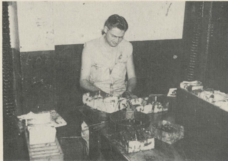
GORMAN WELBORNE , pattern builder for the Weaving department, is shown at the messy job of constructing a chain that governs the designs to be woven on a loom. (Staff Photo)
