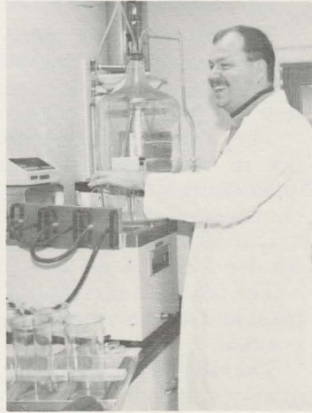
Russ Roach analyzes fabric for "fogging" or "hazing."
