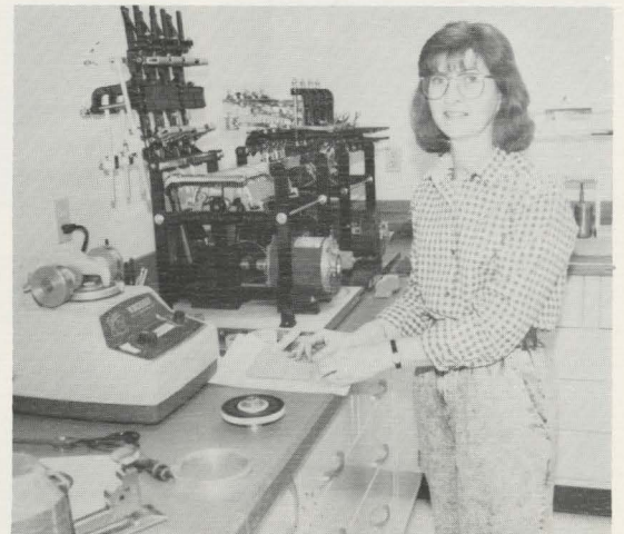
Bonnie Butcher prepares a swatch for the Taber Abrasion tester.
