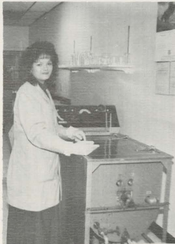
Cindy Haynes prepares to unload the Launderometer to check how a swatch sample has dyed.
