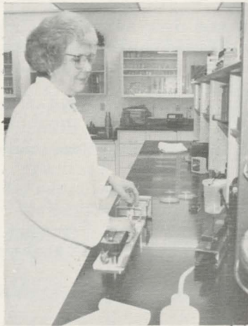
Betsy Lyon tests fabric on the Perspir-ometer, which predicts the effect of perspiration on fabric.
